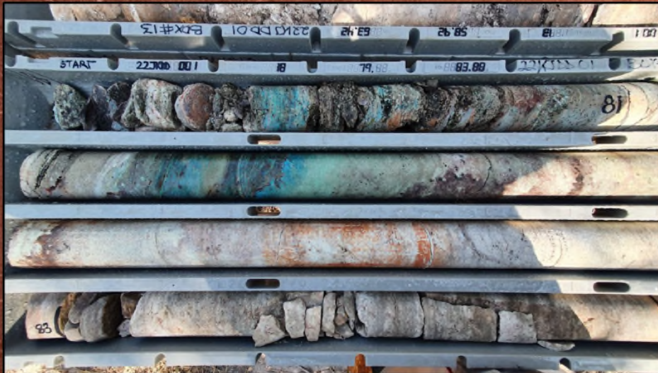
Copper mineralisation in drill core, Jacks Copper Project
